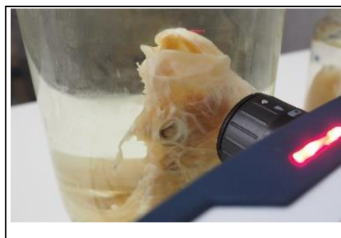
Fig. 1. Portable Raman analysis of wet specimens from the Natural History Collection, Sydney University Museums.
