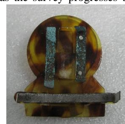
Fig. 1. Cellulose nitrate object with severe corrosion on metal parts.
